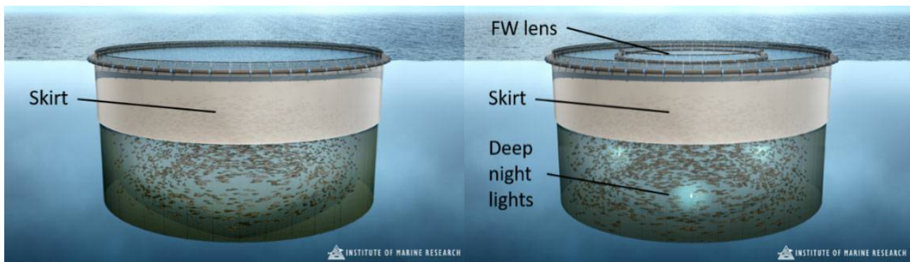
Figure 1. Schematics of a standard skirt cage (left) and a “Well” skirt cage with an additional central FW lens pool, and smart lighting and feeding (right). Drawings revised from Bui et al. (2017). Smart lighting and feeding entails using lights and feed delivery positions to move stock in ways that avoid their exposure to low dissolved oxygen within the skirt and FW lens pool spaces, but also maximise brackish water salinity exposure in the FW lens pool for lice treatment at critical timepoints.
