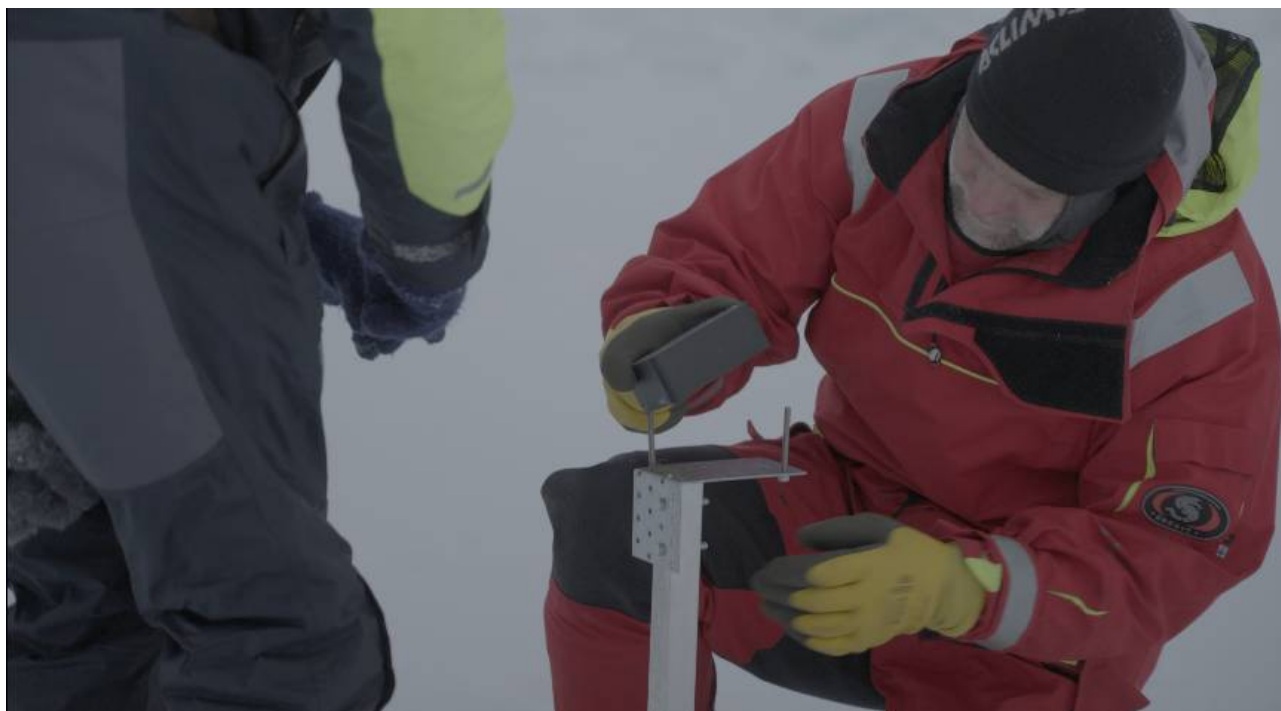
Fig. 4. Deployment of Iridium-linked GPS beacon beacons on an ice floe in the West Ice (Photo: Michael Poltermann).
